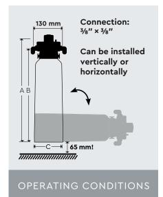
Inlet pressure: 2 - 8 bar Water temperature: 4 - 30 °C Ambient temperature: 4 - 40 °C
